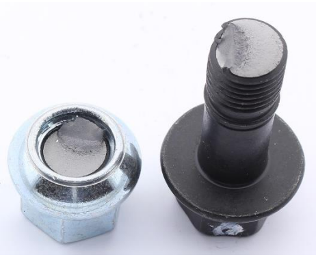
Failure location of Lightweight optimized Bolts
